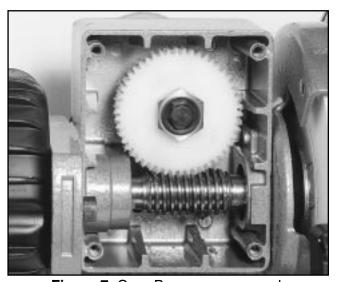
Figure 7. Gear Box cover removed.
